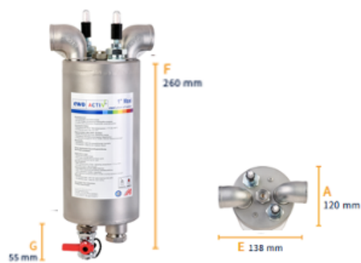
EWO® ACTIV 1" Maxi for 1.000 - 2.500 liters system volume 2 PCS. magnesium anodes
